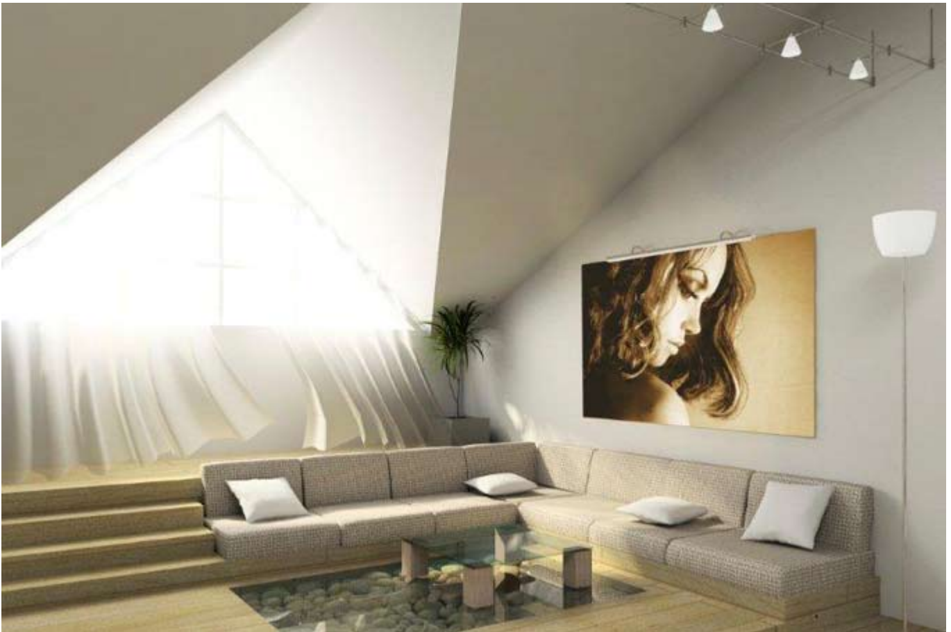
Wire lighting systems are often used in areas where it would be a challenge to mount other types of lighting, such as in rooms with very high ceilings, cathedral or vaulted ceilings and ceilings interrupted by soffits, beams or exposed ductwork.
